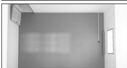
For rooms greater than 25 ft (7.6 m) long or wide, leave an expansion gap of 5/8" (15 mm).
